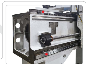
Vertical guideway layout for Y axis
