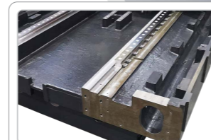
Integrated chip removal groove in casting base
