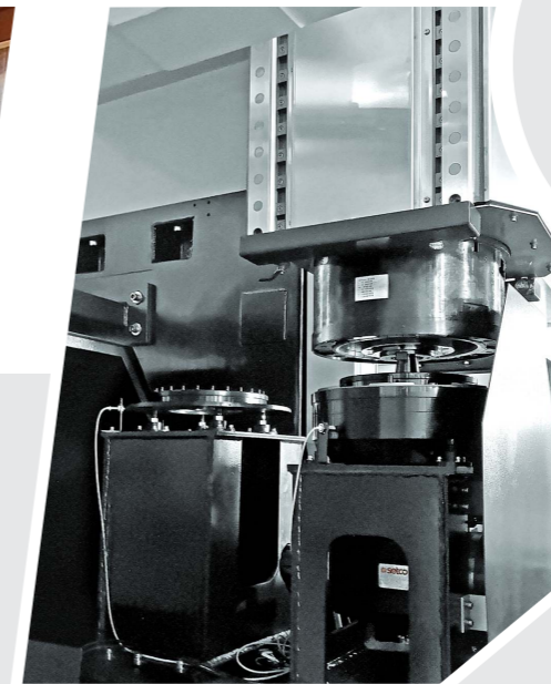
Fully automatic head exchange AAC
